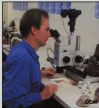
Visual picking: 0.25-0.5, 0.5-1.0, 1.0-2.0 mm fractions
