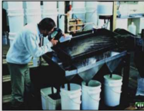
Preconcentrate heavy minerals on shaking table
